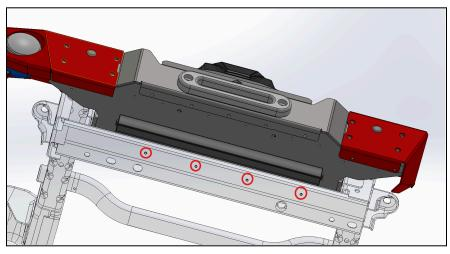
Then simply hold the Splash Guard up under the bottom of the Modular Front Bumper, and install the hardware using (14) M4x16mm Button Head Flange Bolts.
